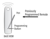
3. Carefully remove front cover of Chronis Timer, and using a paper clip, pen, or similar device, briefly press the programming button on the Chronis Timer until the window covering "jogs".
